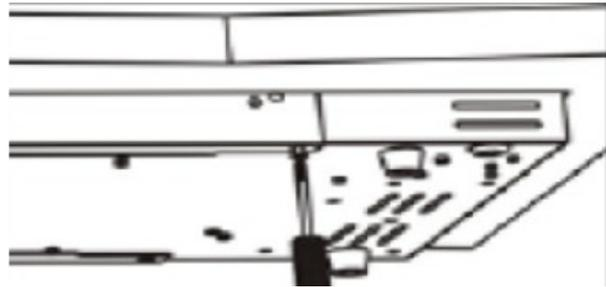
5. Carefully insert the appliance in the built-in structure.
