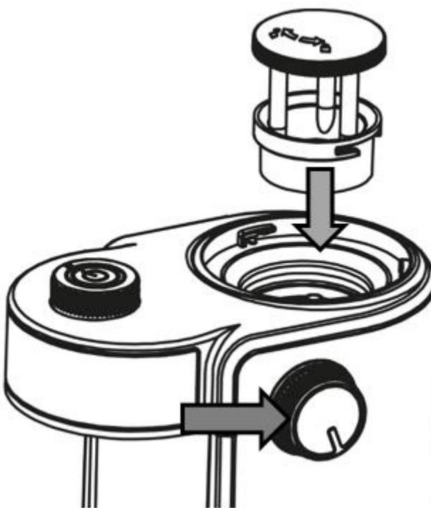
Place the grinder and turn it slightly back and forth so that the grinder will slides down into the guidance
